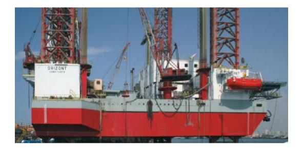
ORIZONT Rig PEMEX Contract No. 421001807: "Lease with no option to purchase the Jack up drilling platform, cantilever type, independent leg with nominal maritime capability to operate in water depth of 300' (three hundred feet) called "GSP ORIZONT" with minimal drilling capacity of 25,000 ' (Twenty five thousand feet) deep including comprehensive maintenance to operate in Mexican waters of the Gulf of Mexico."
